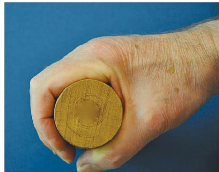
Graspable, circular cross-sectional handrail. (Photo courtesy of Jake Pauls)
